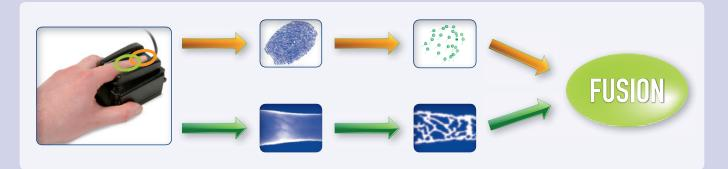
World leader in biometrics, Morpho has developed the first ever multimodal device capable of capturing and processing finger vein and fingerprint biometric data at the same time.
